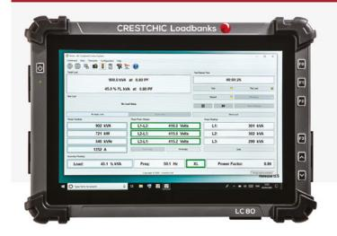
Controlled by either Crestchic's dedicated LC80 rugged tablet controller, or via a standard PC over super-fast, interference free fibre optic cable.
